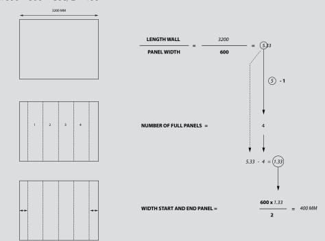
Take into account an expansion joint of 1mm per running metre (maximum 8 metres) and the location of windows and doors. Avoid posts and battens near pipes and other utilities.
